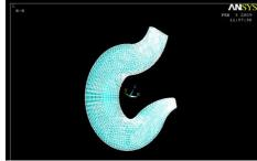
Fig 1 Meshed crane hook
